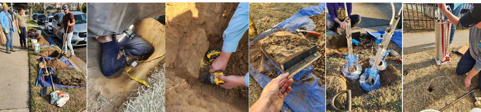
Left-to-Right: 1) Researchers excavating soil pit in parkway; 2) Taylor McDowell photographing soil profile; 3) Preparation of soil monolith; 4) Prepared soil monolith in tray; 5) Unsaturated hydraulic conductivity test; 6) Saturated conductivity test. Photos by Igor Bronz
