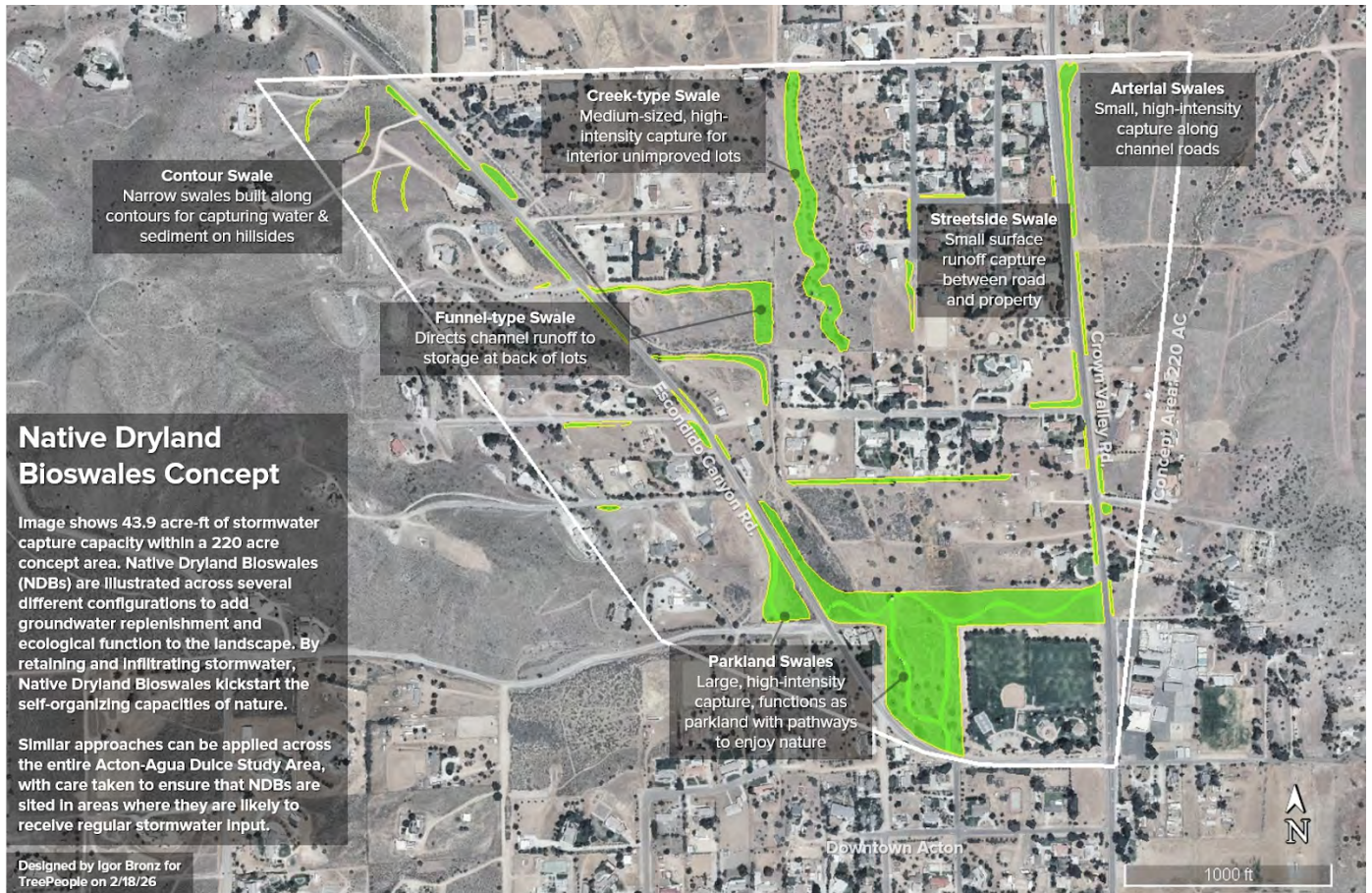
Figure 15: A conceptual drawing of potential locations for various configurations of Native Dryland Bioswales within a 220-acre concept area just north of downtown Acton
