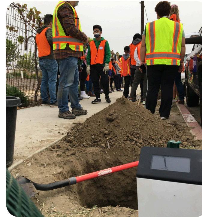
Figure 3 - A vertical soil column excavated for sensor probe installation with a METER Teros datalogger visible in the foreground (left) and sensor probes installed against a vertical soil face at 10, 20, 30 and 50 cm depths (right).
