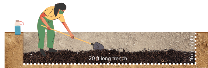
Figure 9 - A compost amendment trench measuring 20 feet length by 16 inches of depth. A 4 inch layer of compost is added to be mixed with the soil that was removed from the trench.
