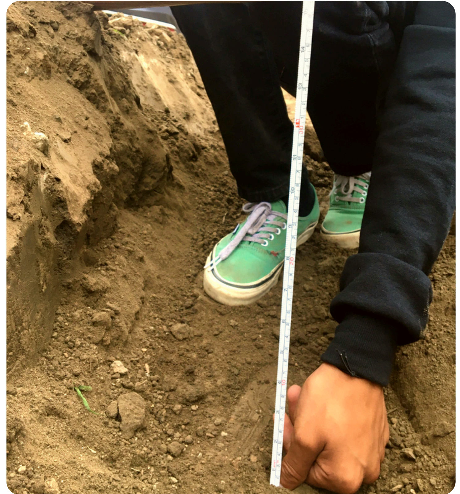
Figure 10 - A study team member measures the depth of an amendment trench prior to mixing in compost.
