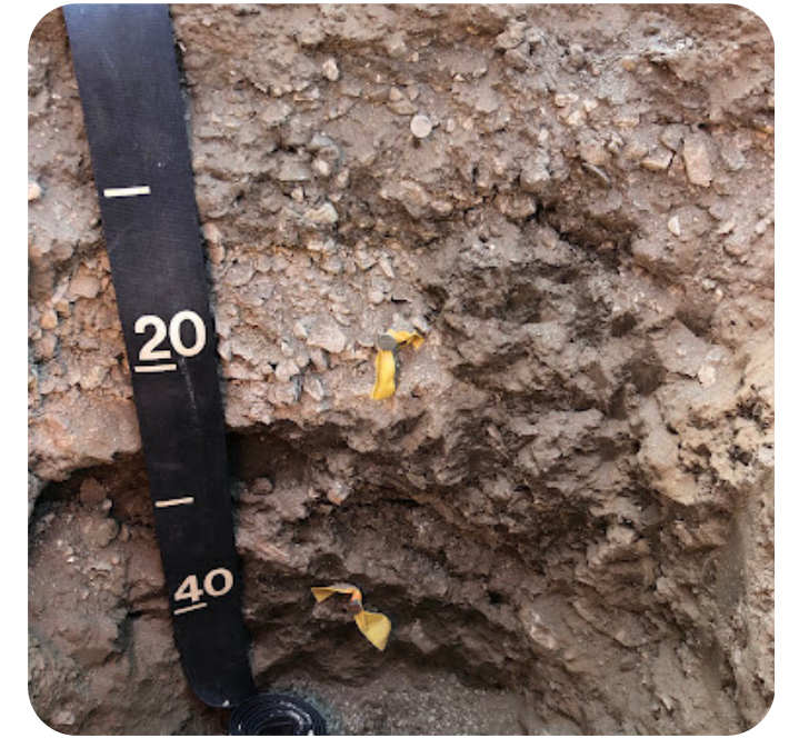
Figure 20 - Site D4 pit with coarse soil texture from gravel and construction backfill visible down to 50 cm.
